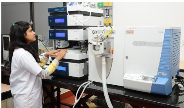
**Tandem LC with ion trap mass analyzer (LC-MS)**
