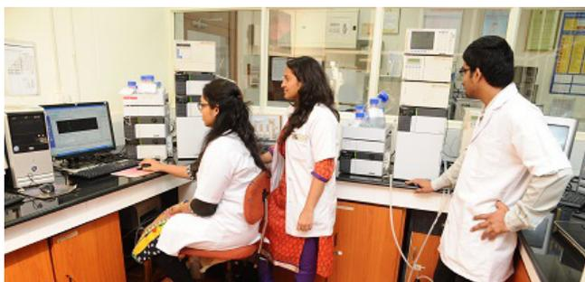
**High-performance liquid chromatography (HPLC systems - various detectors including ECD, UV, PDA and fluorescence)**
