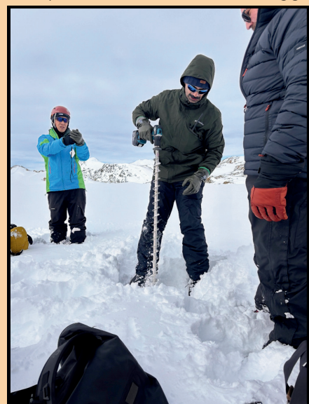
Fig. 3 Dr. Anish Kumar Warriar (MAHE) is drilling through the lake-ice to measure the water depth in Lake Priddy, Stornes Peninsula.
